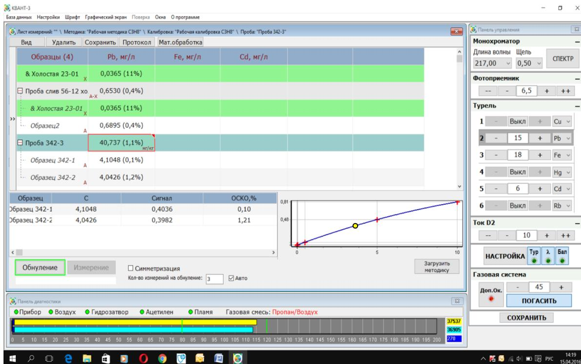
The screenshot displays the Kvant-3 software interface. The main window shows a table of measurement results for lead (Pb), iron (Fe), and cadmium (Cd). The table has columns for 'Образцы (4)', 'Pb, мг/л', 'Fe, мг/л', and 'Cd, мг/л'. The row for 'Проба 342-3' is highlighted in green, indicating it is the active sample. The value for Pb in this row is 40,737 (1,1%).
